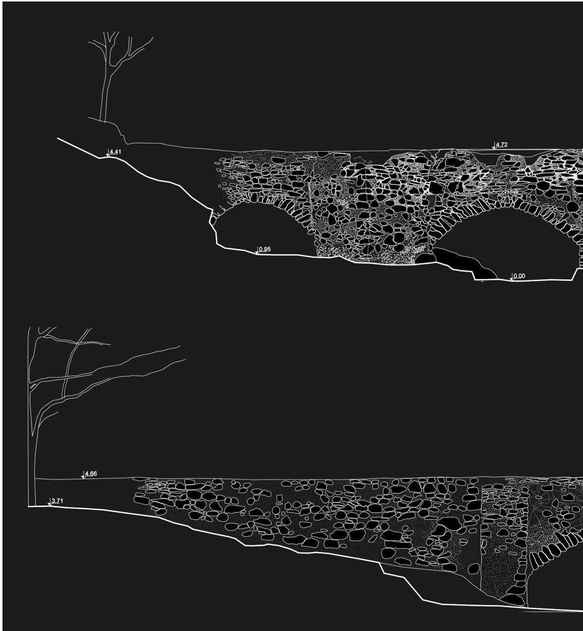
Fig. 6 – North and South elevations of the stone masonry arched Espada aqueduct in San Antonio (Texas). The aqueduct allowed the crossing of the Espada acequia with the natural water feature of Piedras creek (drawing by Ydnechachew Maru's master thesis, 2021).
